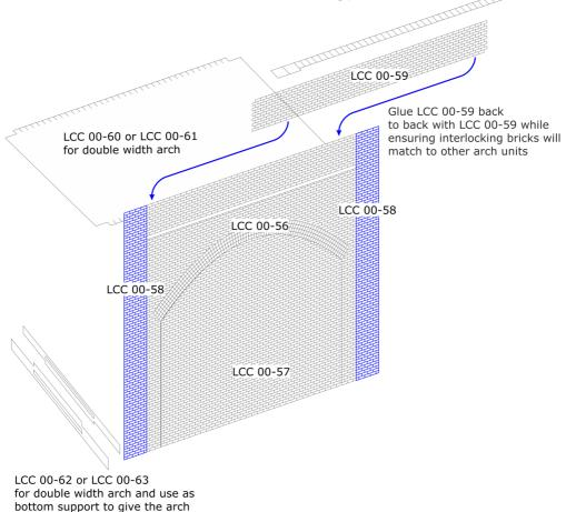
TO ASSEMBLE ARCH UNIT IN LOW RELIEF CONFIGURATION SPLIT LCC 00-60 OR LCC 00-61 IN THE MIDDLE. THIS KIT ASSEMBLED IN LOW RELIEF VERSION CONTAINS ENOUGH PARTS TO MAKE DOUBLE LENGTH ARCH (USE ADDITIONAL LCC 00-58 AND LCC 00-69 PROVIDED).
